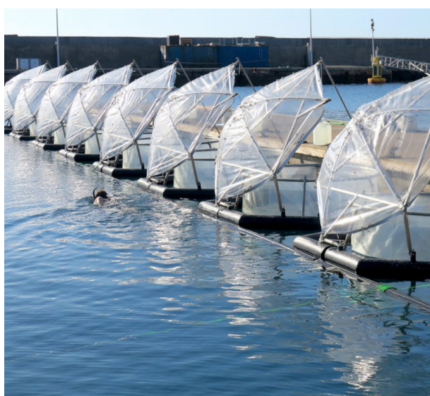
Figure 6: Two mesocosm experiments: on-shore mesocosms (left), employed on Gran Canaria, Spain, and the Off-Shore Mesocosms for Ocean Simulations (KOSMOS), here employed in the Raunefjord nearby Bergen, Norway.
